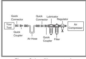
Figure 2. Installing your tool.
